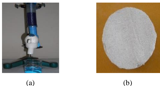
Figure 1 (a) Photograph of experimental filtration unit for the degradation of the methylene blue
